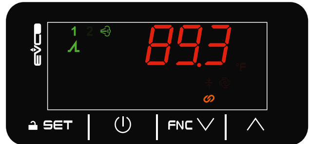
Fig. 31. Proportional operation - ID1 and ID2 closed
