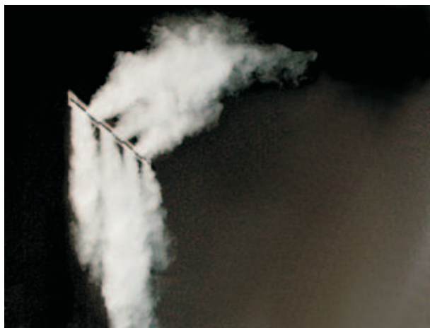
Fig. 4: Jet spread made visible by smoke tracer Above: at an upward incline and downwards Right: horizontal
