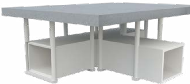
Take-off point on horizontal duct
