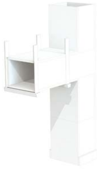
Take-off point on a vertical duct
