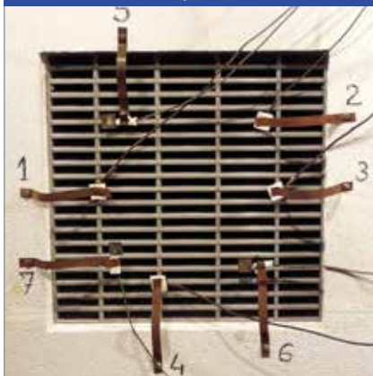
VENTILODICE V before fire resistance test (non-exposed side)
